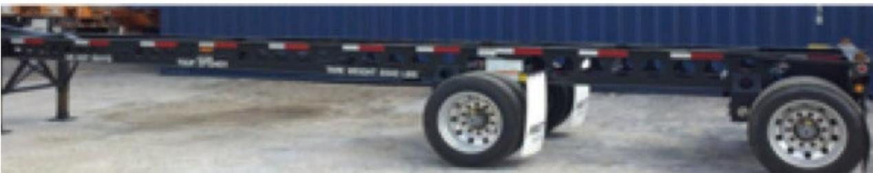
**Figure 2: Slider Chassis**
