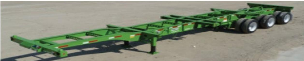
**Figure 3: Triple Axle Chassis**
